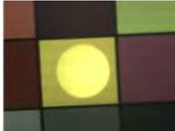
Figure 3. Imaged captured by the Viewfinder Camera showing the precise region of the NED under test which will be measured by the spectroradiometer.
