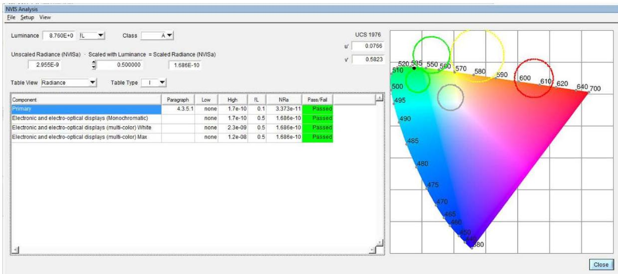
Figure 4. The final NVIS class A analysis results are shown here for the electronic and electro-optical display cockpit component categories.
